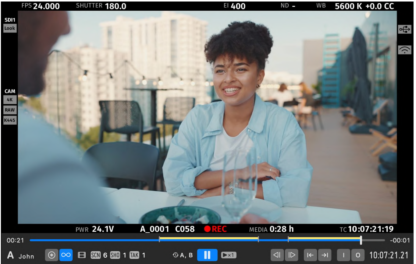
Playback controls with editing options and enabled ranges playback and loop playback
